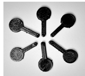
Fig. 4. The 3D printed plastic caps that empower the solenoid plungers to control the fine metal pins' movement such that the user can feel the movements of the six braille pins on his fingertip.
