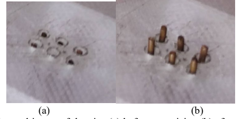
Fig. 7. Zoomed image of the pins (a) before energizing (b) after energizing the solenoids showing the pin height.
